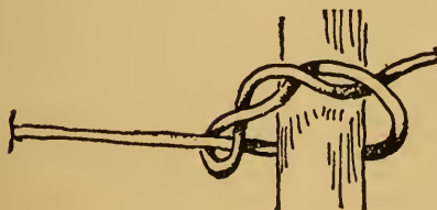
Timber hitch: cannot slip or jam; easily loosed.
