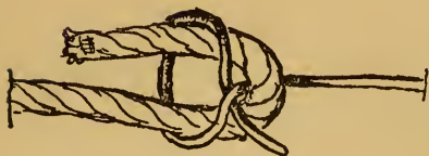
Becket hitch, for joining a cord and a rope.
